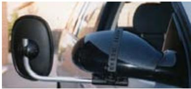
This mirror can be extended and swivelled horizontally and vertically. Easily installed and removed. Clear visibility when towing vans up to 2.4m wide. Easily adjusted from inside car. Sold in pairs. **000962**
