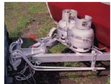
Assists in reducing sway when towing by distributing the weight of the towed vehicle. To calculate which equalizer should be used, add the caravan towball weight to the weight of the luggage in car boot. Note: for weights over 125kg, use a load distribution hitch with suitable rating
