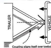
2 piece system fits on the towball as a guide when backing up to the trailer. Suits standard towball and torsion bar fittings. Long shank towballs are recommended when used in conjunction with torsion bar fittings.
