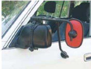
Fits most vehicles, strong and stable, vibration resistant, easily installed and removed. No tools needed. The addition of the suction support arm will prevent any problems drivers sometimes experience with clip-on mirrors. **000969**
